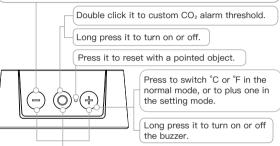
After powering off, long press the 3 buttons to enter calibration mode then the device begins to count down 200s on the screen. Pay attention to doing it outdoors without people.
